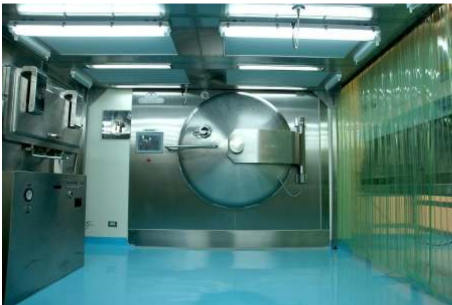
The independent lyophilizer for BCG ampoules
