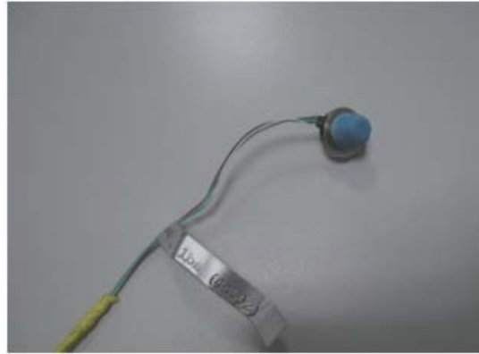
ELFS-B3-2L-R Type: LOAD CELL Range: 2 LBS Temperature Range Compensated: 70 to 170° F Operating: -40 to 250° F Sensor: +In(Red) , -In(Black) , +Out(Green) , -Out(White)
